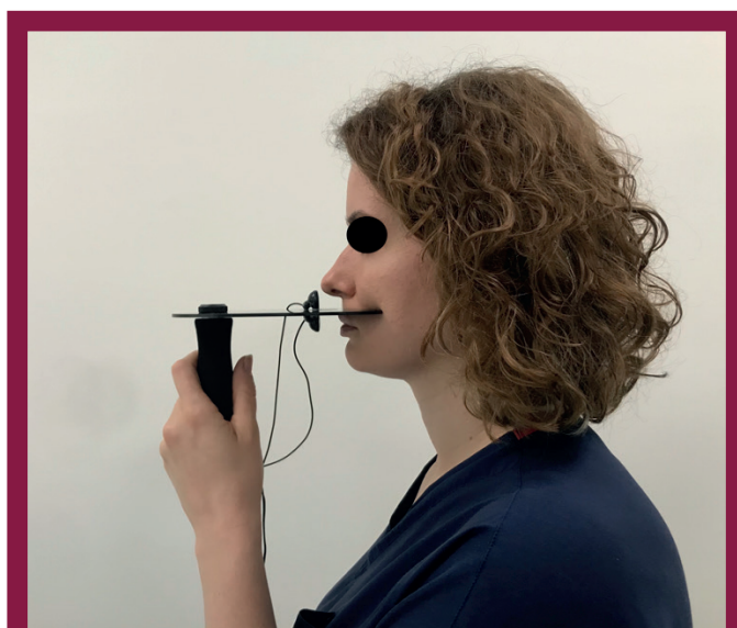
Figure 2. A participant holding a Praat-Assisted Nasalance Meter device above the vermilion border. The edge that comes into contact with the upper lip is concave so that there is no gap in between. There is a small line showing the middle line with an oval hole 21 mm away from this edge so that microphones can be easily placed in the appropriate position. The second hole at the other end of the plate with a diameter of 7 mm is for the handle to be mounted.
