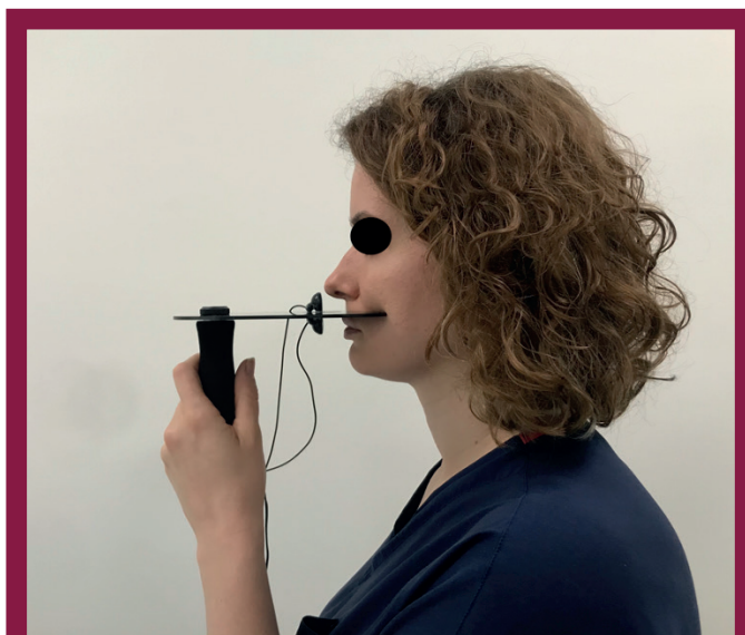
Figure 2. A participant holding a Praat-Assisted Nasalance Meter device above the vermillion border. The edge that comes into contact with the upper lip is concave so that there is no gap in between. There is a small line showing the middle line with an oval hole 21 mm away from this edge so that microphones can be easily placed in the appropriate position. The second hole at the other end of the plate with a diameter of 7 mm is for the handle to be mounted.
